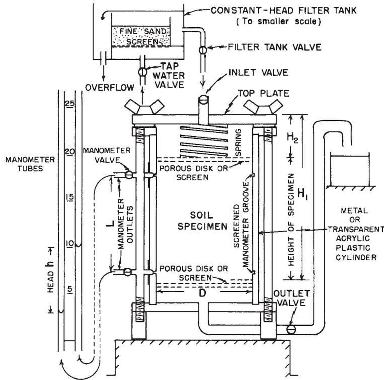
FIG. 1 Constant-Head Permeameter
