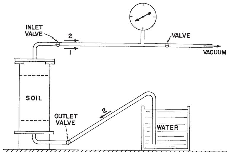
FIG. 2 Device for Evacuating and Saturating Specimen
