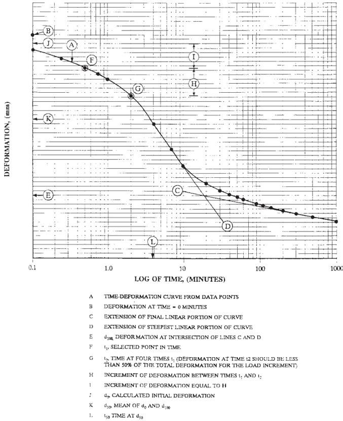
FIG. 2 Time-Deformation Curve From Log of Time Method
