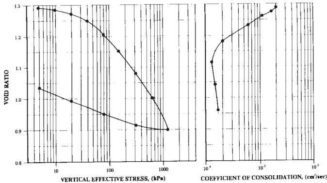
FIG. 5 Example of Consolidation Test Summary Plots
