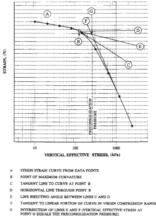
FIG. 4 Evaluation for Preconsolidation Pressure From Casagrande Method
