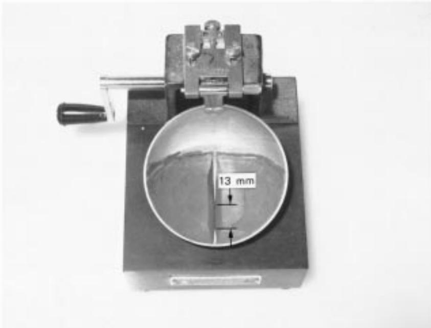
**FIG. 7 Soil Pat After Groove Has Closed**
