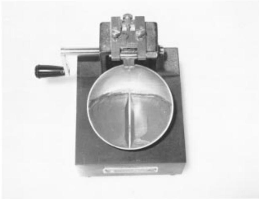
**FIG. 6 Grooved Soil Pat in Liquid Limit Device**
