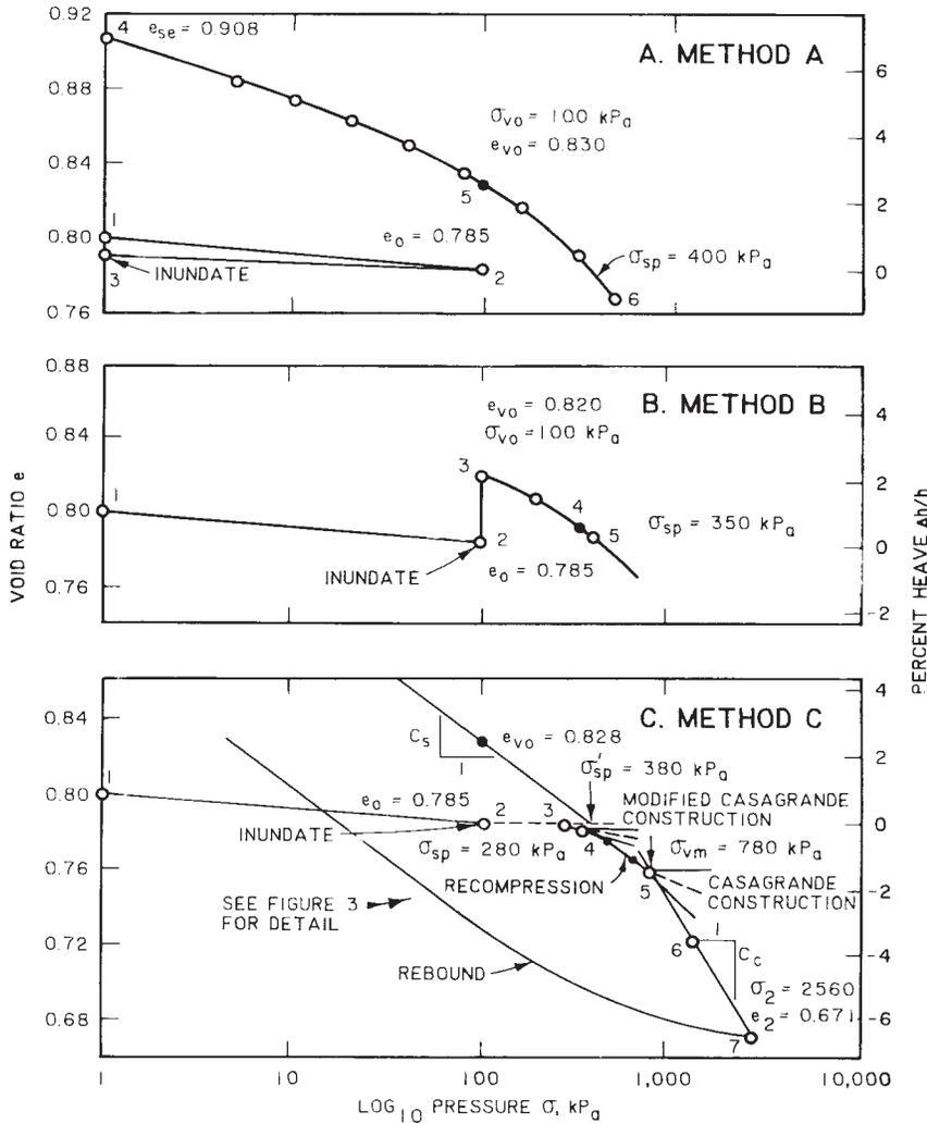
FIG. 2 Void Ratio - Log Pressure Curves
